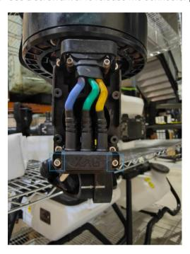
03 Use a screwdriver to release the 3 screws that tighten the connectors and check the insulator and connector hub condition.
